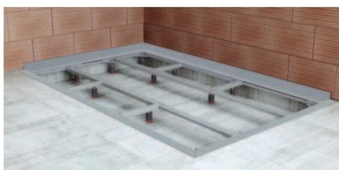
LE CADRE EST CONFORME AUX EXIGENCES DE LA NORME DIN 4109 "ISOLATION PHONIQUE DES BÂTIMENTS", GRÂCE À SES NOMBREUX POINTS D'ISOLATION: PIEDS MULTIPLES AVEC TALON ISOLANT, PROFILÉ EN CAOUTCHOUC CELLULAIRE ET BANDE POLYÉTHYLÈNE.
